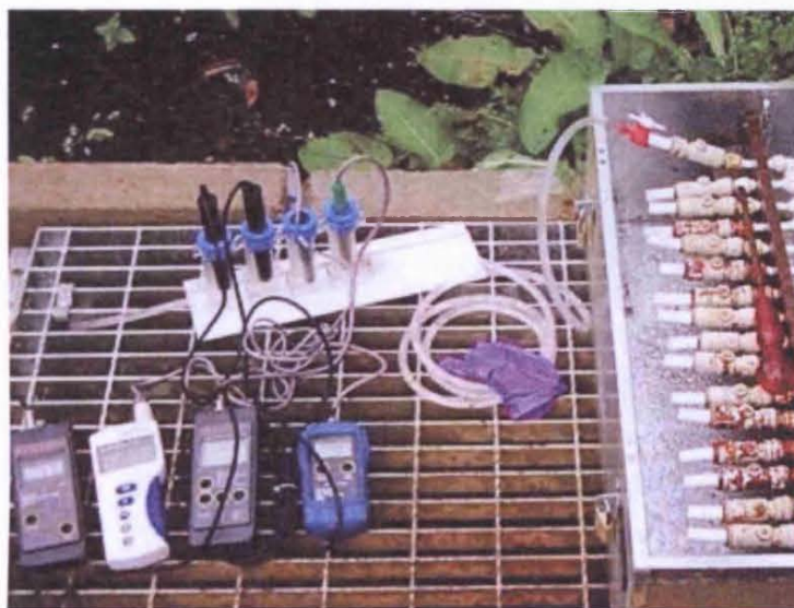
Figure 5-2: VFR sample port monitoring using a Waterra Sheffield flow through cell and hand held meters
