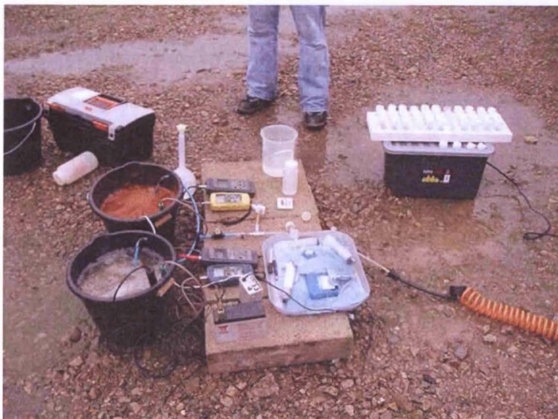
Figure 5-5: Fe(II) oxidation rates being determined in the field
